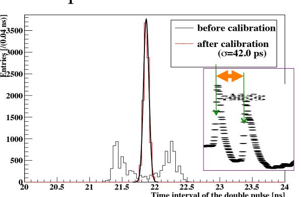
time difference of two test pulses
