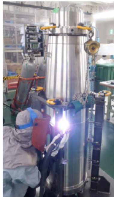
Covering the cold mass with the helium vessel and welding the vessels
