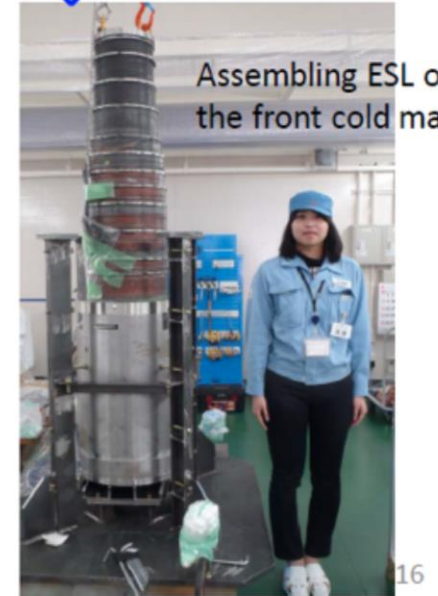
Assembling the radiation shield of W alloy on ESL
